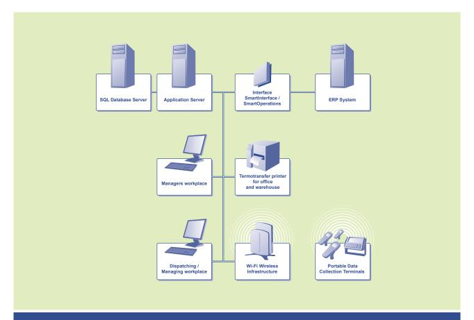
img.1 SmartStock.WMS System Architecture
